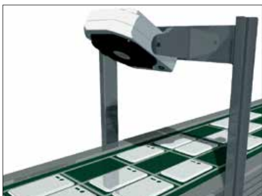
Dust prevention on molded parts
