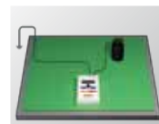
Resistance between a ground and a connecting point by a probe on a surface
