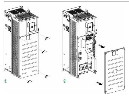
Apply the following instructions to access the terminals on **frame sizes 4 and 5** drives
