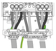
PA/+ and PB terminals are used to connect a braking resistor. Refer to the braking resistor instruction sheet NHA87388 available on www.se.com.
