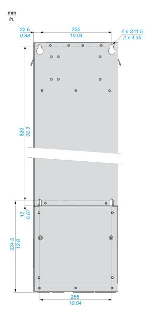
**NOTE:** Lower Conduit Box part VW3A9704 sold separately. This part enables wall mounting of the product. It provides IP21 protection degree on the lower part and UL type 1 protection degree.
