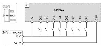
Switch set to **EXT** (Sink External) position **with functional isolation** on digital inputs. This configuration requires the use of 2 external supply units.
