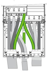
PA/+ and PB terminals are used to connect a braking resistor. Refer to the braking resistor instruction sheet NHA87388 available on www.se.com.
