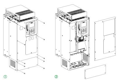
Apply the following instructions to access the terminals on **frame sizes 3S and 5S** drives
