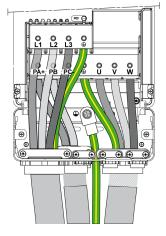
PA/+ and PB terminals are used to connect a braking resistor. Refer to the braking resistor instruction sheet NHA87388 available on www.se.com.
