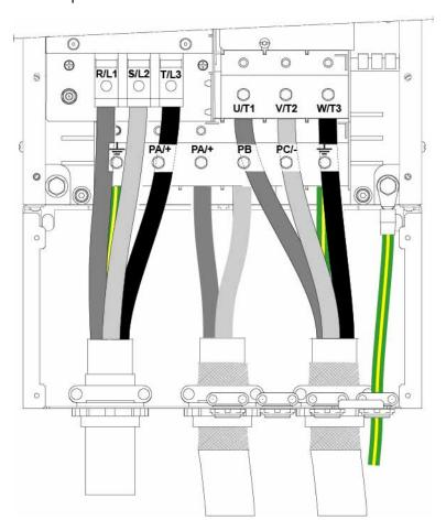
PA/+ and PB terminals are used to connect a braking resistor. Refer to the braking resistor instruction sheet NHA87388 available on www.se.com.
