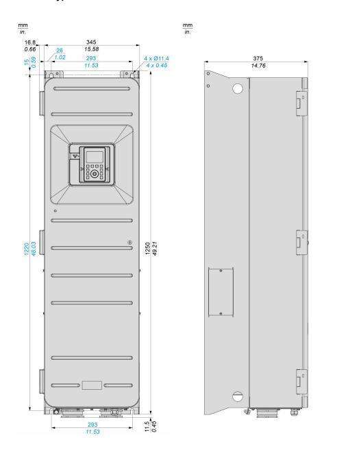
IP55 / UL Type 1 Drive With Disconnect Switch - Front and Side view
