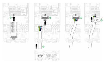
**NOTE:** Cabling plate shown is for frame size 2. Other cabling plates look slightly differs from this one.
