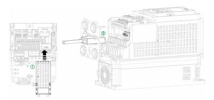
To help ensure correct wiring of the control part, apply the following instructions to install the PROFIBUS fieldbus module on Frame size 1 drives
