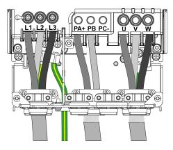
PA/+ and PB terminals are used to connect a braking resistor. Refer to the braking resistor instruction sheet NHA87388 available on www.se.com.
