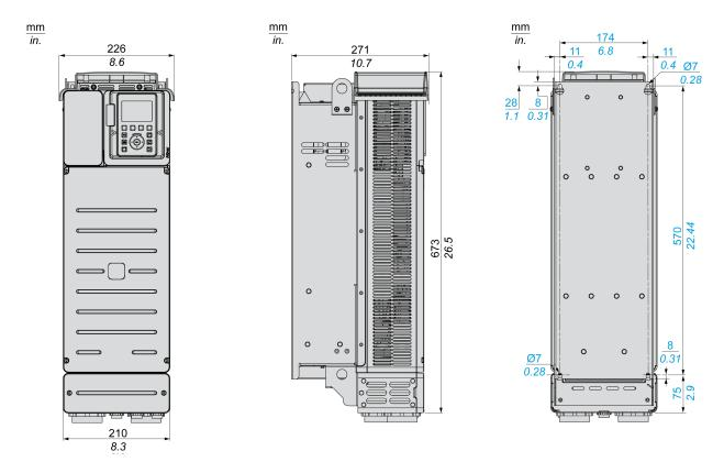
IP20 Drives, except on Lower Part side (IP00) - Front, Side And Rear View
