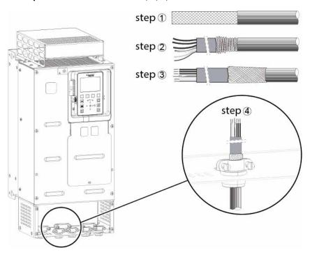
Example for drive frame sizes 4, 5, 5S, 5Y, 6, 7 and FSP
