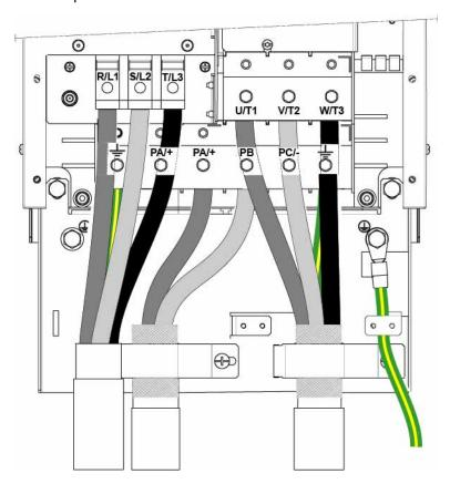
PA/+ and PB terminals are used to connect a braking resistor. Refer to the braking resistor instruction sheet NHA87388 available on www.se.com.
