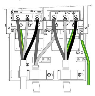
PA/+ and PB terminals are used to connect a braking resistor. Refer to the braking resistor instruction sheet NHA87388 available on www.se.com.
