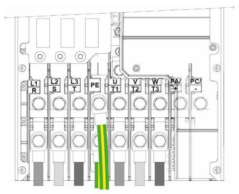
**NOTE:** PA/+ and PC/- terminals are used to connect the braking unit. Refer to the braking unit instruction sheet NVE16635 available on www.se.com.
