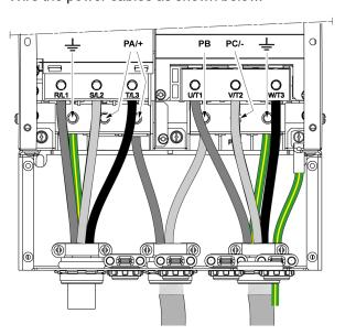
PA/+ and PB terminals are used to connect a braking resistor. Refer to the braking resistor instruction sheet NHA87388 available on www.se.com.
