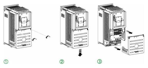
Apply the following instructions to access the terminals on **frame sizes 1 to 3** IP20 drives
