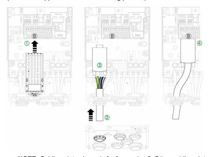
**NOTE:** Cabling plate shown is for frame size 2. Other cabling plates look slightly differs from this one.
