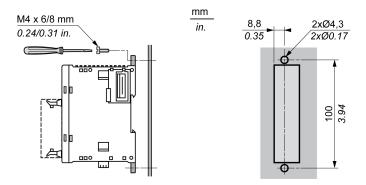
The following diagram shows the mounting hole layout for TM3 with 24 screw or spring I/O channels:
