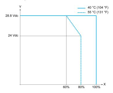
At an ambient temperature of 55  $^{\circ}$ C (131  $^{\circ}$ F) in the horizontal mounting direction, limit the inputs and outputs, respectively, which turn on simultaneously as indicated by the X axis.
