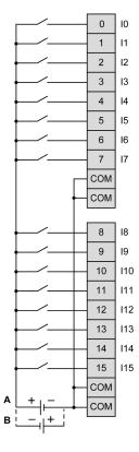
The 4 COM terminals are connected internally
