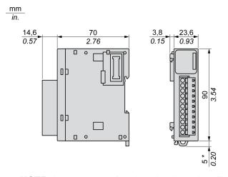
NOTE: \* 8.5 mm (0.33 in) when the clamp is pulled out.
