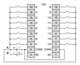
The COM0 terminals are connected internally
