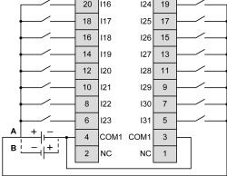
The COM0 and COM1 terminals are not connected internally
