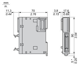
NOTE: \* 8.5 mm (0.33 in) when the clamp is pulled out.
