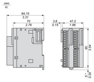
NOTE: \* 8.5 mm (0.33 in) when the clamp is pulled out.
