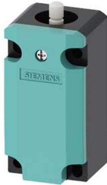
Basic switch for position switch 3SE51 Metal enclosure, according to EN 50041 Device connection 1 x (M20 x 1.5) 1 NO/1 NC quick action contacts without actuator head
