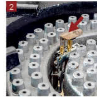
Pilot with cover Prevent pilot extinguish away from drips or liquid
